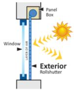
Mounted on the exterior, rollshutters block the sun before it reaches your window. The air trapped between the rollshutter curtain and the window creates another layer of insulation. Both contribute significantly to reducing the cooling energy demand.
